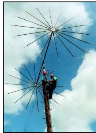
Figure 6—The author adjusting an earlier fiberglass version of his 40-meter Quadruple Cross. Center frequency was 7.2 MHz. The “wheel” diameter was only 14 feet. In contrast, a full-size 40-meter quad would require a diameter of 49 feet.
