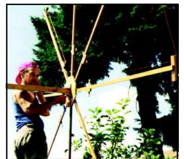
Figure 7—At left, a cedar version of the 20-meter Double Cross quad at VE7FJR just before it was installed. Above, Dave, VE7DWG, assembles the quad elements to the boom.
